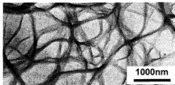
Figure 3. Transmission electron micrograph of 1 in chloroform. Sample is post stained by uranyl acetate.
